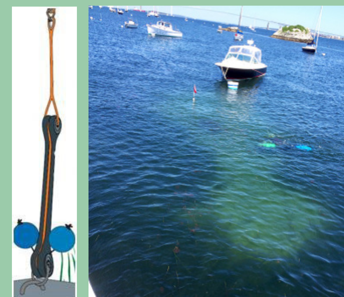
Fig. 5 Hazelett mooring system. (left)
