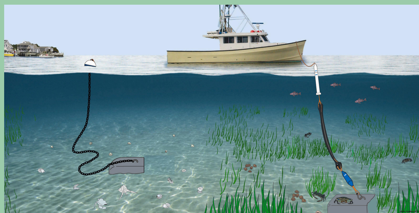
Fig. 1 Traditional moorings (left) create a halo of bare substrate whereas conservation moorings (right) allow for seagrass to thrive.
