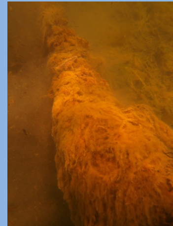
Figure 6. Fouled mooring dragging the bottom.
